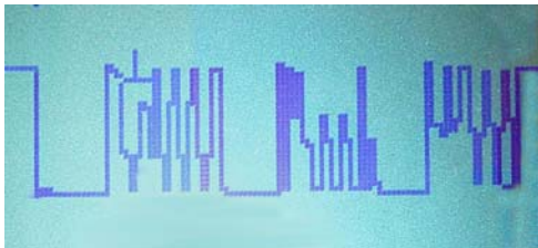
Figure 16: 100 kHz Digital Scope CAN Waveform
