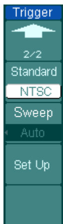
Figure 2-41 Table 2-22 The Video Trigger menu (When the Sync is set as All lines, Odd field and Even field)
