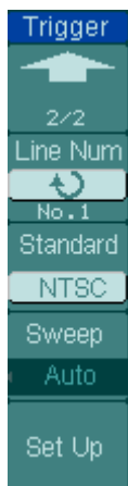
Figure 2-40 Table 2-21 The Video Trigger menu (Page 2/2, when Sync is set as the specified line)
