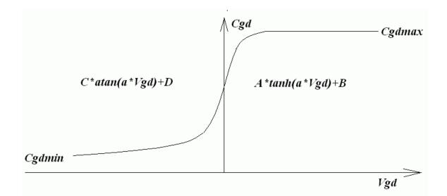
For positive Vgd, Cgd varies as the hyperbolic tangent of Vgd. For negative Vdg, Cgd varies as the arc tangent of Vgd. The model parameters a, Cgdmax, and Cgdmax parameterize the gate drain capacitance. The source-drain capacitance is supplied by the graded capacitance of a body diode connected across the source drain electrodes, outside of the source and drain resistances.
