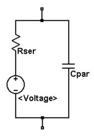
Voltage sources have historically been used as the current meters in SPICE and are used as current sensors for current-controlled elements. If Rser is specified, the voltage source can not be used as a sense element for F, H, or W elements. However, the current of any circuit element, including the voltage source, can be plotted. Syntax: Vxxx n+ n- PULSE(V1 V2 Tdelay Trise Tfall Ton Tperiod Ncycles )
