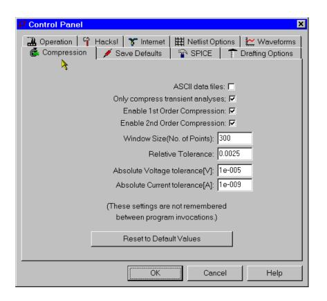
LTspice compresses the raw data files as they are generated. A compressed file can be 50 times smaller than the un-compressed one. This is a lossy compression. This pane of the control panel allows you to control how lossy the compression runs.
