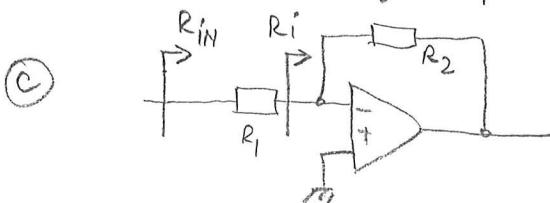
Use Eq. 6.23  $\Rightarrow R_{IN} = R_1 + R_i = R_1 + \frac{R_2}{1 + \omega_0} \cdot \frac{1 + j \frac{f}{f_B}}{1 + j \frac{f}{f_t}} \Rightarrow$
