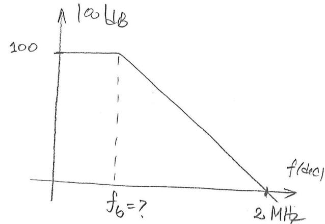
$$\textcircled{b} \quad A_o = 10 \quad , \quad f_t = A_o \cdot f_B \quad \Rightarrow \quad f_B = \frac{f_t}{A_o} = 200 \text{ kHz.}$$
