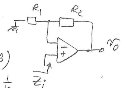
$$f = 500 \text{ kHz} \Rightarrow |Z_i| = R_{id} \cdot \left| \frac{1 + j \frac{f/f_B}{f/f_b}}{1 + j \frac{f/f_B}{f/f_b}} \right|$$
