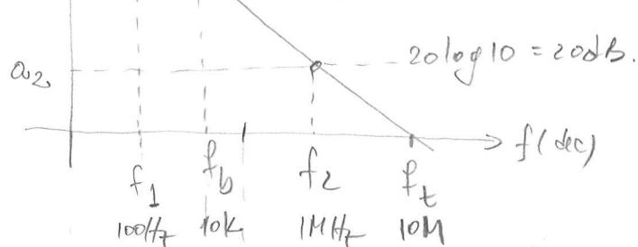
$$\text{GBP} = f_t = \alpha_f \cdot f = \omega_2 \cdot f_2 = 10 \cdot 1 \text{ MHz} = \boxed{10 \text{ MHz} = f_t}$$
