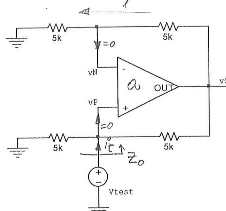
$$i_t = \frac{V_{\text{test}}}{R} + \frac{V_{\text{test}} - V_O}{R} = \frac{V_{\text{test}} + V_{\text{test}} - 2V_N}{R} = \frac{2}{(1 + \frac{a}{2})R} \cdot V_{\text{test}} \Rightarrow$$
