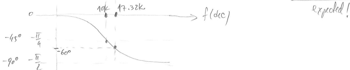
$$(b) |\alpha(jf)| = \frac{\omega_0}{\sqrt{1 + \left(\frac{f}{f_b}\right)^2}} \Bigg|_{f=f_x} = 2 \frac{\text{V}}{\text{V}} \Rightarrow \left(\frac{\omega_0}{2}\right)^2 = 1 + \left(\frac{f_x}{f_b}\right)^2$$
