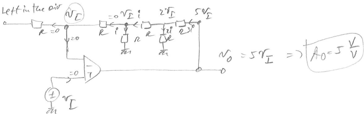
$$A_0 = 5 \text{ V/V} \quad \beta = \frac{1}{5} \Rightarrow G_{BP} = 4 \text{ MHz.}$$
