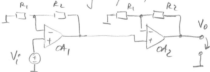
$$\text{Gain } A_1 = 1 + \frac{R_2}{R_1} \quad \text{Gain } A_2 = 1 + \frac{R_2}{R_1} : \text{make them equal for maximum bandwidth!!!}$$
