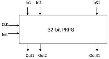
The PRPG should have the capability of seed loading. This is done by holding *Init* high in the first clock cycle. When *Init* is high, the PRPG is loaded with values from the inputs. *Init* becomes and remains low from the second clock cycle on. Starting from the second clock cycle, the PRPG generates a random 32-bit vector every clock cycle. Use the following generating polynomial to design the structure of the circuit:
