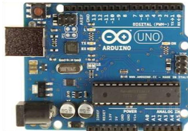
Figure 1: Arduino Uno board.
