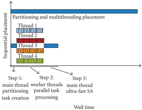
FIGURE 5: Illustration of Step 2. Sixteen tasks are processed concurrently by four worker threads (see also Figure 3). This step exploits parallelism to achieve overall speedup.
