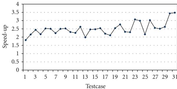
FIGURE 7: Illustration of the speedup variation proportional to the circuit size. The first circuit on the  $x$ -axis is the smallest and the last one is the largest.
