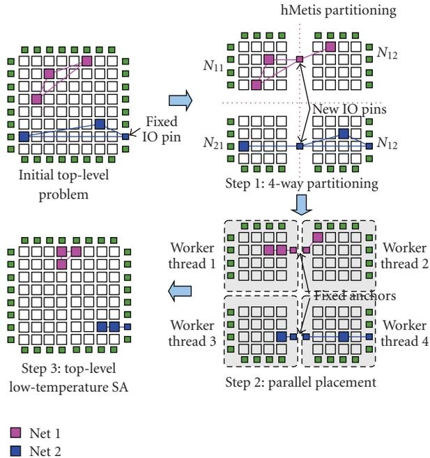
FIGURE 4: Subchip *new IO pins* are created during partitioning. They will act as fixed anchors during the parallel placement of all subchips.
