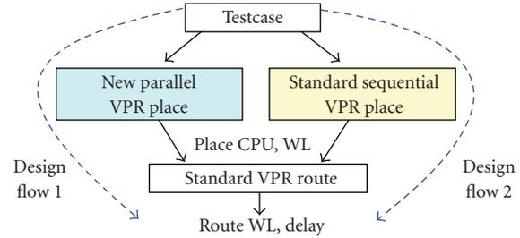
FIGURE 6: The flow diagram of the experimental setup with two design flows: first design flow uses the proposed parallel VPR placement algorithm and the second design flow uses the standard sequential VPR placement algorithm.
