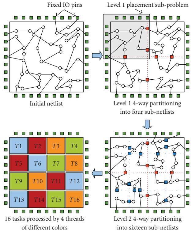
FIGURE 3: Illustration of Step 1. The FPGA is decomposed into multiple balanced regions using multilevel 4-way partitioning. These regions represent tasks to be processed concurrently.
