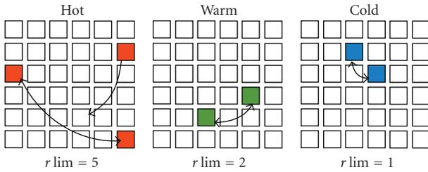
FIGURE 2: Illustration of how  $r_{lim}$  controls moves inside the SA-based placement algorithm of VPR [12]. Initially, at high temperatures, blocks far away from each other can be easily swapped. Finally, at low temperatures, only blocks close to each other can be swapped.
