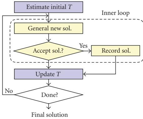
FIGURE 1: Block diagram of the classic simulated annealing (SA).
