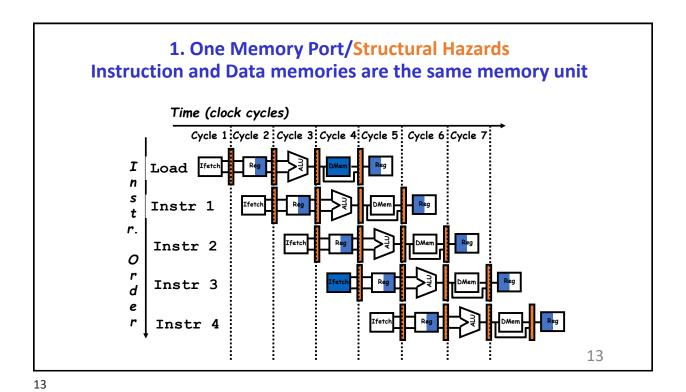
**Structural Hazards** Time (clock cycles) Cycle 1 Cycle 2 Cycle 3 Cycle 4 Cycle 5 Cycle 6 Cycle 7 Load Ifetch Ι n S Instr 1 r. Instr 2 0 r STALL e Instr 3 How do you "bubble" the pipe? De-assert all control lines in 14 appropriate pipe stages.
