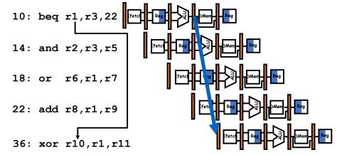
If we had to wait until the end of EX state to find out if branch is taken or not taken (untaken); Let's assume it's taken; What do you do with the 3 instructions in between? We need to STALL (i.e., do nothing or delay, NOP) the pipeline 3 stages now or FLUSH (i.e., discard) later.
